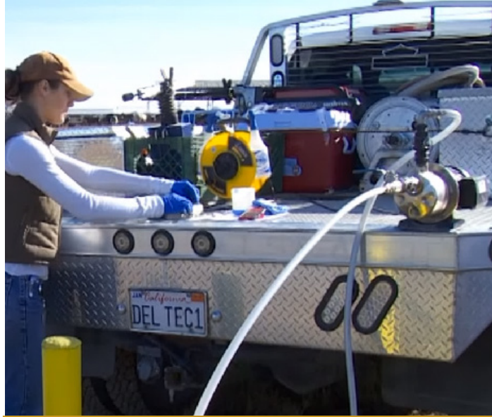
A CVDRMP well is sampled to measure depth to first-encountered groundwater, total dissolved solids, nitrogen and general minerals.
